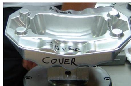
Applying High-Speed Machining to a calliper part results in excellent surfaces.
