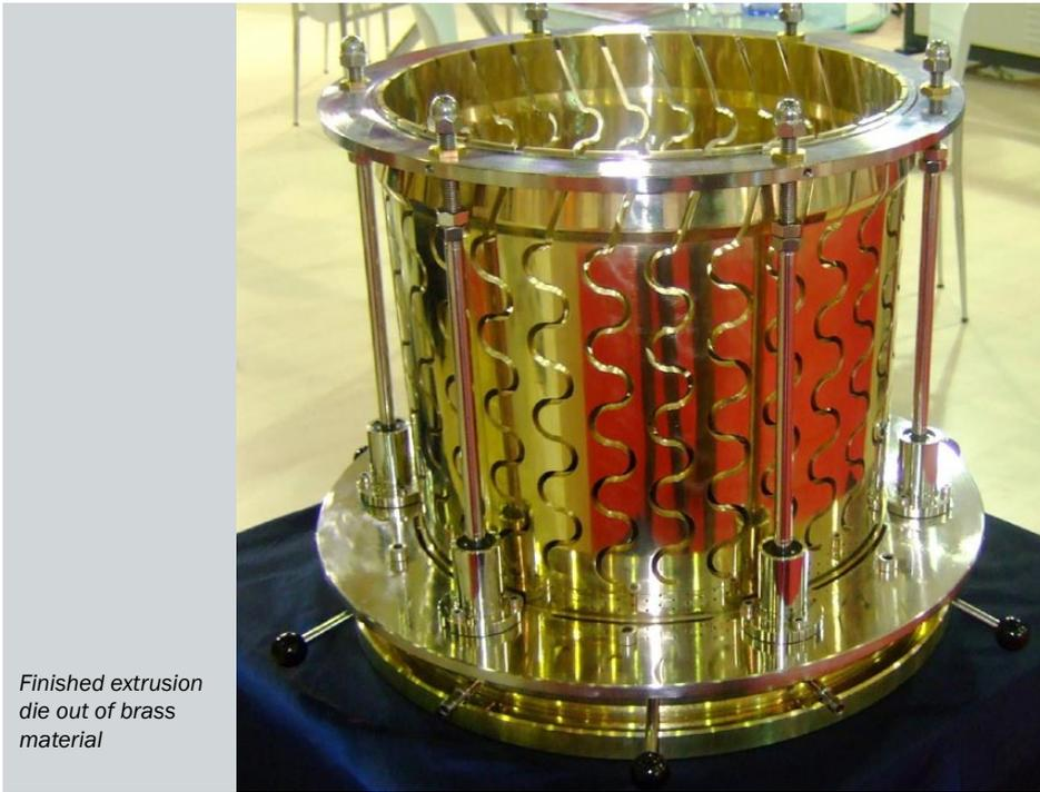
Finished extrusion die out of brass material
