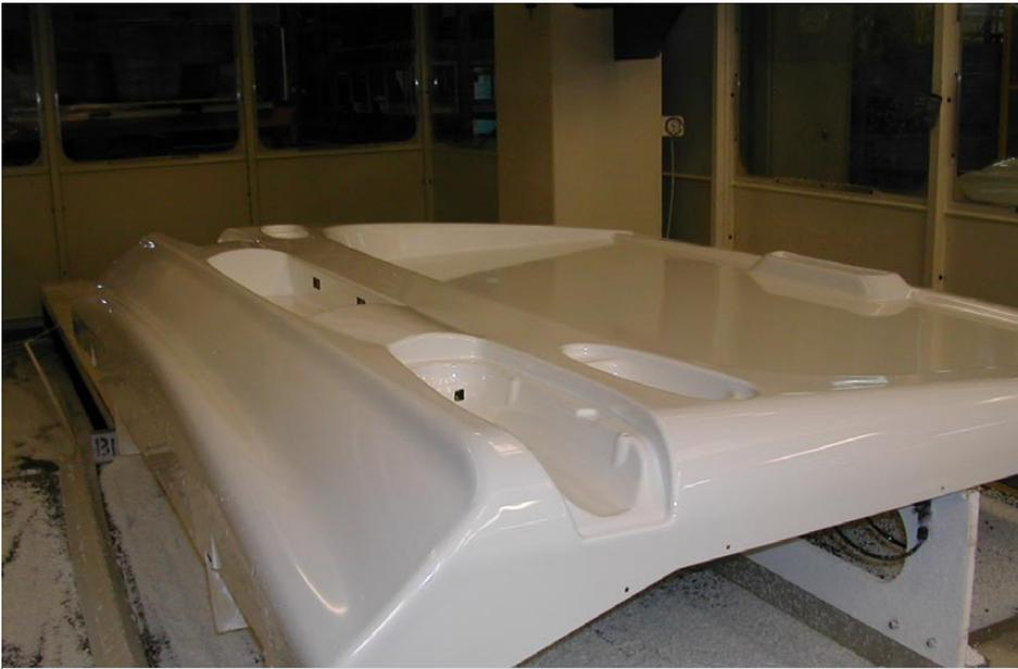
Finished panel after trimming has been performed
