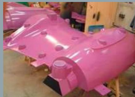
Wooden model of one half of the ship drive – produced by Jozsko Modele
