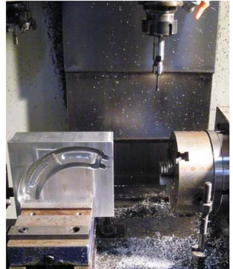
*Finished component of a surgical instrument to place implants*
