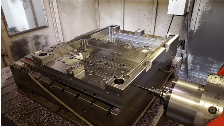
*Manufacturing a part of a plastic pressing mold using Trimill HF2012 seven-axis CNC machine tool. Photo: Marek Pagáč*
